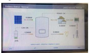
**Step7:**Make the inverter start charging battery to 100% to calibrate SOC.
