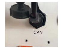
**INV-BAT**: From the master box CAN IN to the inverter CAN port;
