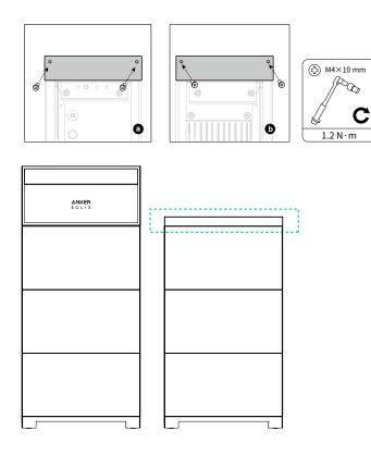
4. Install the base baffles when installing two columns of modules.
