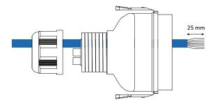
3 Insert the wires into the RJ45 connector (included) in the EIA/TIA 568B order. From left to right (when the clip is facing away from you):
