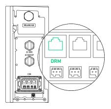
2 Route a signal cable (Cat 5 or higher, 5-6 mm in diameter, not included; shielding recommended) through the locking cap and wiring compartment cover. Then, strip the insulation layer.
