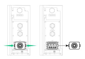
Remove the wiring compartment cover by pressing the clips on both sides.
