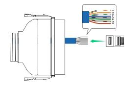
• Crimp the RJ45 connector using a crimping tool. Ensure that the pins click in place.
