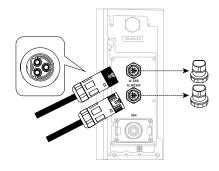
Connect the AC grid connector to the home main panel, and the AC backup connector to the sub panel.
