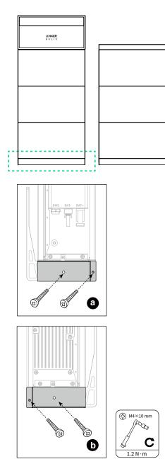
Figure: Install the base baffles for wall mounting.
