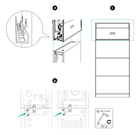
if necessary, insert the included wedge shim into the power module's mount bracket to ensure stability.
