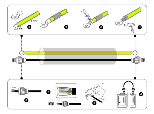
3 Install the GND cable and RJ45 signal cable.
