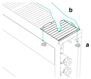
**2** Open the WLAN/4G port cover on the right side of the power module.
