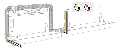
(2) Assemble the GND cable and RJ45 signal cable.
