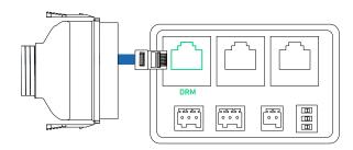
Connect the other end of the signal cable to the Demand Response Enabling Device (DRED).
