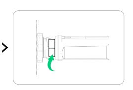
OPress the back of the panel to reinstall it, and then tighten the screws (M3×8 mm).
