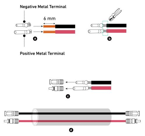
(5) Install the positive and negative DC power cables.
