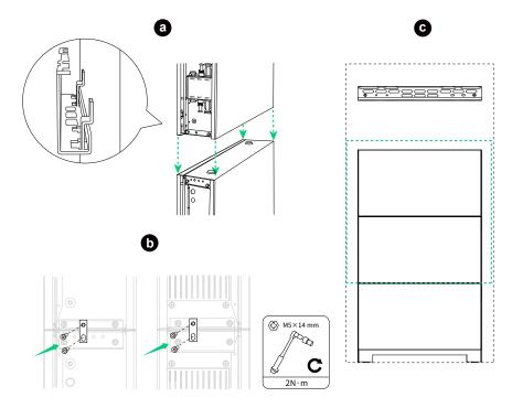
Figure: Mount the power module.
