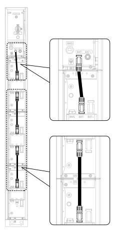
6. Connect the positive DC power cables between the modules.
