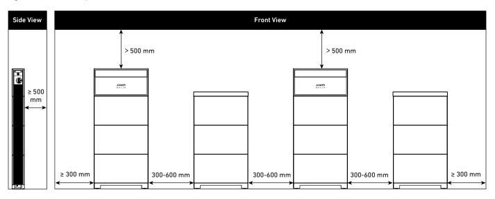
Figure: Installation space for wall-mounted modules.
