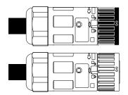
Route the 3-conductor cable (6 mm<sup>2</sup>, not included) through the nut, claw, seal body, and body. Strip the insulation layers from the conductors, and insert and crimp the tube terminals.
