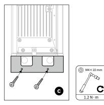
Figure: Install the base baffles for floor mounting.
