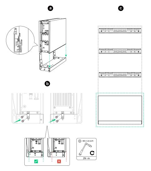
2 Mount the remaining modules from bottom to top. After installing a module, tighten the module interlockers using the screws (M5×14 mm, included), and then mount the next module.
