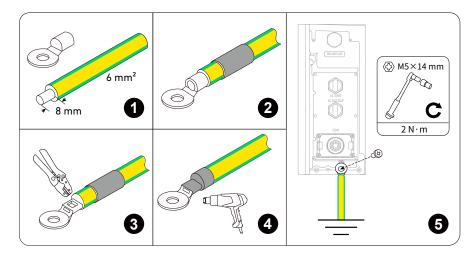
3. Connect the GND cables between the modules.
