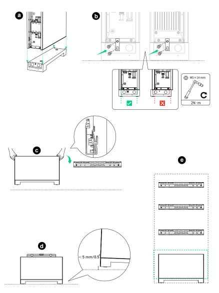
2 Mount the remaining modules from bottom to top. After installing a module, tighten the module interlockers using the included screws (M5×14 mm), and then mount the next module.
