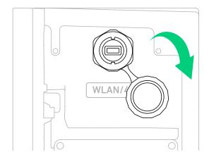
Install the appropriate dongle according to the networking methods.
