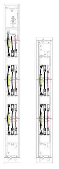
3. Connect cables between the bottom modules.
