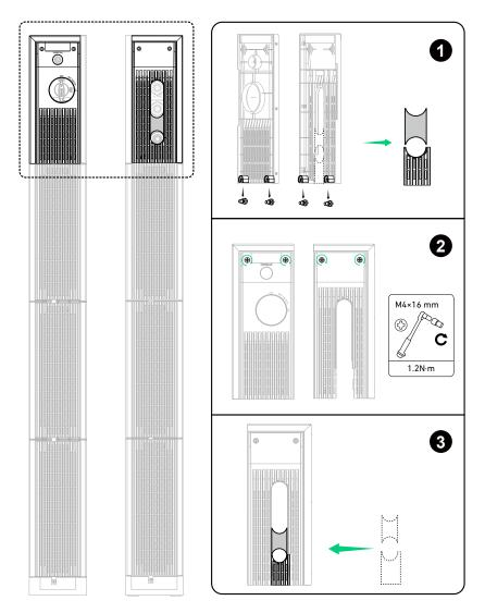
3. Install the top cover baffles when installing two columns of modules. Figure: Install the top cover baffles.
