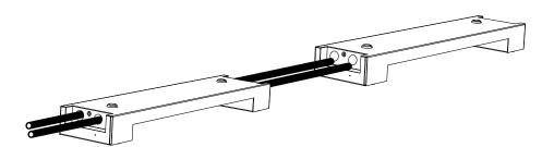
For **wall mounting**, route cables from the back of the first column into the second column. Figure: Conduit run for wall mounting.
