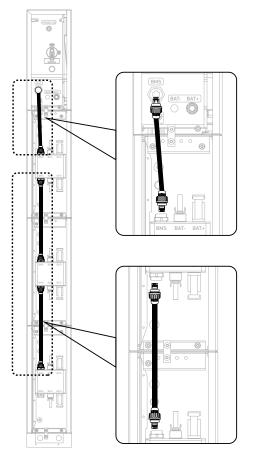
5. Connect the negative DC power cables between the modules.
