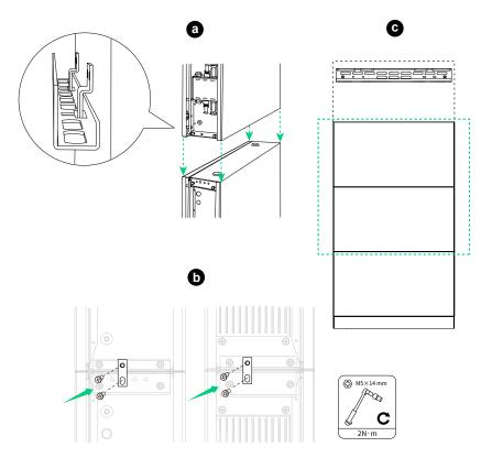
Figure: Mount the power module.
