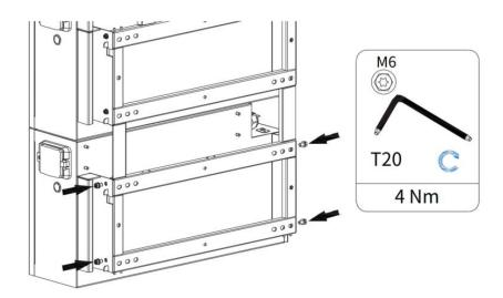
Step 8: Remove the rubber plugs from the top battery, and remove the screws on the cover of batteries with T20 screwdriver.
