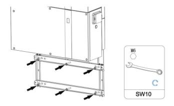
Step 6: Hold the handles on both sides of the battery pack and install the battery pack on the wall bracket. At least, two people are required for this step.
