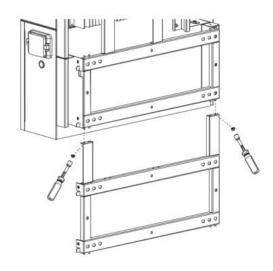
Step 4: Mark the positions according to holes on the bracket and remove the assembled wall bracket.
