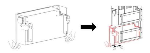
Step 7: Tighten the wall bracket and the battery pack with screw M6\*16 (X4) (tool: T20 screwdriver, torque: 3.0 Nm).
