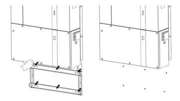
Step 5: Attach the expansion bracket to the wall by tightening the screws with SW10 hexagon sleeve.
