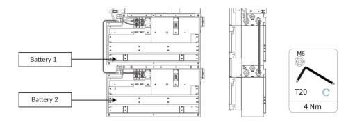
Step 11: Connect the BMS communication cable from battery 2 to battery 1.
