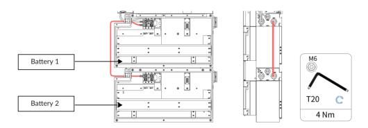
Step 10: Connect the negative power cable from battery 2 to battery 1 (tool: T20 screwdriver, torque: 3 Nm).
