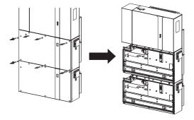
10. Remove the cable box cover by unscrewing the screws at the top of the inverter by hand and perform electrical connection work (please refer to Chapter 7.7).
