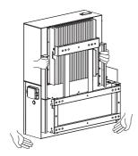
5. Tighten the wall bracket and SMILE-B3-PLUS with screw M6\*16 (X6) (tool: T20 screwdriver, torque: 3.0 Nm).
