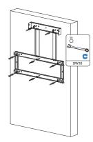
4. Hold the handles on both sides of the inverter and install SMILE-B3-PLUS on the wall bracket. This step should take two people to complete.
