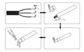
5. Fix the terminals with different color conductors on the corresponding electrode holders, and use a #2 Phillips screwdriver to tighten them one by one with a torque of 2 Nm.
