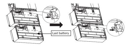
Connect the positive power cable from battery 2 to battery 1 (tool: T20 screwdriver, torque: 3 Nm).
