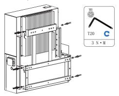
6. Install the holders for cable box cover (tool: T20 screwdriver, torque: 2.5 Nm)
