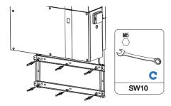
7. Hold the handles on both sides of the battery pack and install the battery pack on the wall bracket. This step should take two people to complete. (Please install the expansion battery by pushing it from the side)
