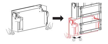
8. Tighten the wall bracket and the battery pack with screw M6\*16 (X4) (tool: T20 screwdriver, torque: 3.0 Nm).
