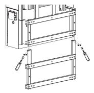
6. Attach the wall bracket for expansion to the wall by tightening the screws with SW10 hexagon sleeve.
