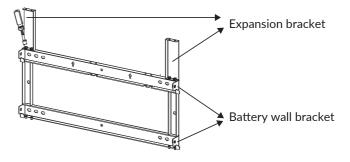
Use two M4 flange nuts to fix the wall bracket assembled in the step 1 to the wall bracket of SMILE-B3-PLUS (tools: SW7 sleeve or other tools for M4 flange, torque: 1.6 Nm).
