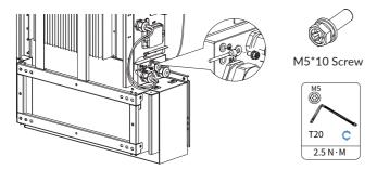
Connect the expanded battery to the ground point of SMILE-B3-PLUS with the grounding cable.
