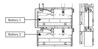
5. Assemble front cover and side cover of the expanded battery with 3 M4 flange nuts (tools: SW7 sleeve or other tools for M4 flange, torque: 1.6 Nm).
