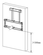
2. Drill 8 holes on the wall with  $\Phi 10$ mm drill and insert 8 screw anchors into the drill holes.
