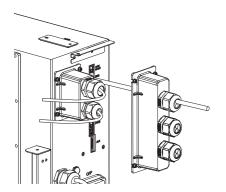
Installation method of two communication cables via M25 cable gland
