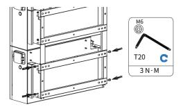
9. Remove the rubber plugs from the battery, and then remove the front cover after unscrewing screws with T20 screwdriver.
