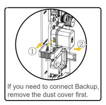
Disassemble the grid or backup plug connector (e.g. due to faulty assembly), proceed as follows:
