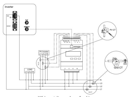
Wiring at three-phase feed in
