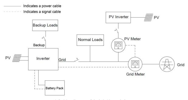
Brief wiring diagram of the hybrid-coupled system
