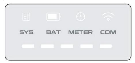
The upper four LED indicators are provided on the display panel. These LED indicators provide information about the operation status of the system.
