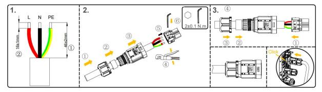
The above wiring steps are both suitable for gird and backup connection. The only difference is that the backup port is already blocked with a cover. If you want to connect the backup connector, please first remove the cover by the tool included in the package.
