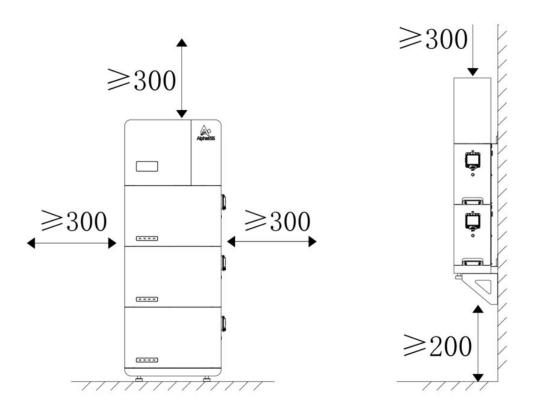
Local Standards may add additional clearance requirements, particularly regarding clearances between the Battery System and other Electrical Appliances.
