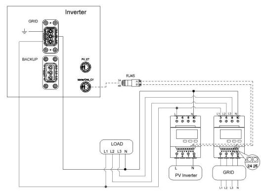
Wiring at three-phase feed in
