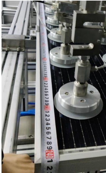
Fig. 11: view of mechanical load mounting
