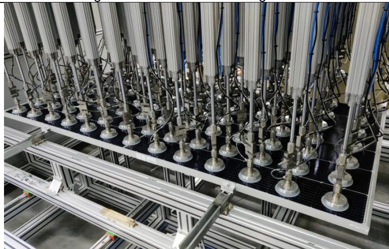
Fig. 14: view of mechanical load mounting
