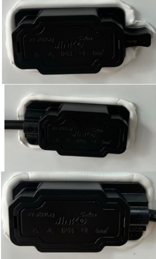
Fig. 79: detail view of closed junction box
