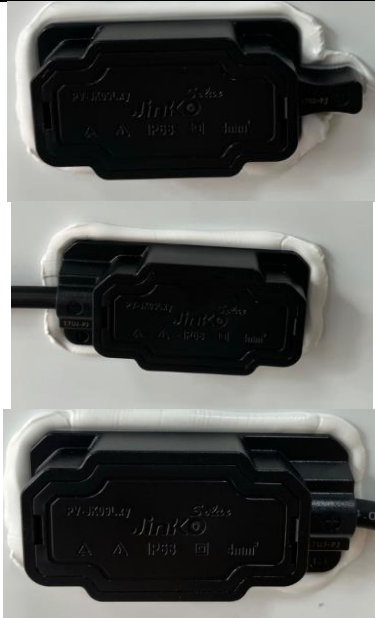
Fig. 60: detail view of closed junction box
