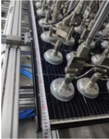
Fig. 85: detail view of mechanical load mounting
